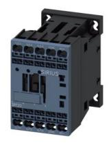
power contactor, AC-3e/AC-3, 12 A, 5.5 kW / 400 V, 3-pole, 24 V DC, auxiliary contacts: 1 NC, spring-loaded terminal, size: S00, communication-capable
