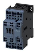
power contactor, AC-3e/AC-3, 38 A, 18.5 kW / 400 V, 3-pole, 220 V AC, 50 Hz / 240 V, 60 Hz, auxiliary contacts: 1 NO + 1 NC, spring-loaded terminal, size: S0
