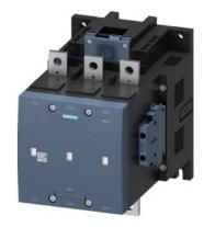
vacuum contactor AC-3e/AC-3 400 A, 200 kW / 400 V, 3-pole, Uc: 96-127 V AC(50-60 Hz) / DC PLC input 24 V DC drive: electronic auxiliary contacts 2 NO + 2 NC main circuit: busbar control and auxiliary circuit: screw terminal
