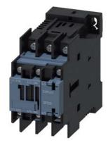
traction contactor, AC-3e/AC-3, 32 A, 15 kW / 400 V, 3-pole, 24 V DC, 0.7-1.25  $^{\star}$  Us, electronic drive, with integrated varistor, auxiliary contacts: 1 NO + 1 NC, ring cable lug connection, size: S0
