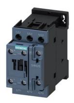
power contactor, AC-3e/AC-3, 32 A, 15 kW / 400 V, 3-pole, 42 V AC, 50 Hz, auxiliary contacts: 1 NO + 1 NC, screw terminal, size: S0
