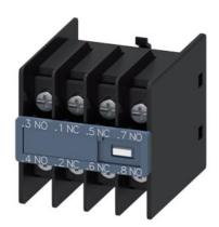
auxiliary switch, on the front, 2 NO + 2 NC, 11 U, .3/.4, .1/.2, .5/.6, .7/.8, current path: 1 NO, 1 NC, 1 NC (lagging), 1 NO (leading), ring cable lug connection, for contactors 3RT2 and contactor relays 3RH2
