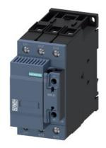
capacitor contactor, AC-6b 50 kVAr, / 400 V, 3-pole, 230 V AC, 50 Hz, auxiliary contacts: 1 NO + 1 NC, screw terminal, size: S2  $\,$
