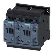
reversing contactor assembly, AC-3e/AC-3, 25 A, 11 kW / 400 V, 3-pole, 230 V AC, 50/60 Hz, screw terminal, electrical and mechanical interlock, auxiliary contacts: 2 x 1 NO
