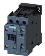
power contactor, AC-3e/AC-3, 17 A, 7.5 kW / 400 V, 3-pole, 24 V DC, with plugged-in diode combination, auxiliary contacts: 1 NO + 1 NC, screw terminal, size: S0
