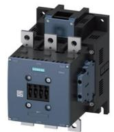
power contactor, AC-3e/AC-3 300 A, 160 kW / 400 V, AC (50-60 Hz) / DC Uc: 440-480 V 3-pole, auxiliary contacts 2 NO + 2 NC drive: conventional main circuit: busbar control and auxiliary circuit: screw terminal
