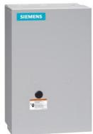
Mechanically held lighting contactor, Contactor amp rating 100A, 0 N.C. / 2 N.O. poles, 24VAC 60HZ coil, Non-combination type, Enclosure NEMA type 1, Indoor general purpose use
