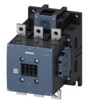
power contactor AC-1 400 A / 690 V / 40  $^\circ$ C 3-pole, Uc: 500-550 V AC(50-60 Hz) / DC drive: conventional auxiliary contacts 2 NO + 2 NC main circuit: busbar control and auxiliary circuit: screw terminal
