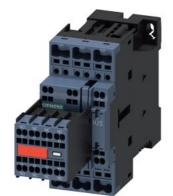
power contactor, AC-3e/AC-3, 32 A, 15 kW / 400 V, 3-pole, 24 V DC, with pluggedin diode combination, auxiliary contacts: 2 NO + 2 NC, spring-loaded terminal, size: S0, captive auxiliary switch
