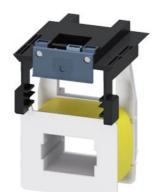
Changeover operating mechanism for contactors 3RT107, 3RT147, AC (50...60 Hz) / DC operation, 21 ... 27.3 V Operating mechanism: electronic with PLC input 24 V DC Screw terminal
