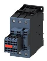
power contactor, AC-3e/AC-3, 80 A, 37 kW / 400 V, 3-pole, 20-33 V AC/DC, 50/60 Hz, with integrated varistor, auxiliary contacts: 2 NO + 2 NC, main circuit: screw terminal, control and auxiliary circuit: spring-loaded terminal, size: S2, captive auxiliary switch
