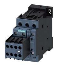
power contactor, AC-3e/AC-3, 25 A, 11 kW / 400 V, 3-pole, 24 V DC, auxiliary contacts: 2 NO + 2 NC, screw terminal, size: S0, removable auxiliary switch
