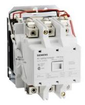
Mechanically held lighting contactor, Contactor amp rating 100A, 0 N.C. / 4 N.O. poles, 208VAC 60HZ coil, Non-combination type, Enclosure NEMA type (open), No enclosure
