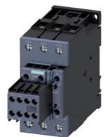
power contactor, AC-3e/AC-3, 65 A, 30 kW / 400 V, 3-pole, 230 V AC, 50/60 Hz, auxiliary contacts: 2 NO + 2 NC, screw terminal, size: S2, removable auxiliary switch
