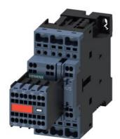
power contactor, AC-3e/AC-3, 38 A, 18.5 kW / 400 V, 3-pole, 24 V DC, with plugged-in diode combination, auxiliary contacts: 2 NO + 2 NC, spring-loaded terminal, size: S0, captive auxiliary switch
