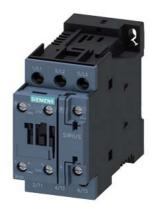
power contactor, AC-3e/AC-3, 17 A, 7.5 kW / 400 V, 3-pole, 24 V DC, with plugged-in varistor, auxiliary contacts: 1 NO + 1 NC, screw terminal, size: S0
