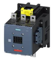
power contactor, AC-3e/AC-3 500 A, 250 kW / 400 V AC (50-60 Hz) / DC 96-127 V x (0.8-1.1) F-PLC input 24 V DC 3-pole, auxiliary contacts 2 NO + 2 NC permanently mounted drive: electronic main circuit: busbar control and auxiliary circuit: screw terminal
