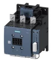
power contactor, AC-3e/AC-3 300 A, 160 kW / 400 V, AC (50-60 Hz) / DC Uc: 96-127 V PLC input 24 V DC 3-pole, auxiliary contacts 1 NO + 1 NC drive: electronic main circuit: busbar control and auxiliary circuit: screw terminal with remaining lifetime indicator
