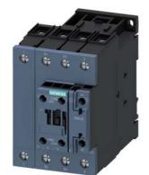
power contactor, AC-3, 51 A, 22 kW / 400 V, 4-pole, 83-155 V AC/DC, 50/60 Hz, with integrated varistor, main contacts: 2 NO + 2 NC, auxiliary contacts: 1 NO + 1 NC, screw terminal, size: S2
