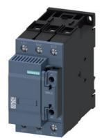
capacitor contactor, AC-6b 50 kVAr, / 400 V, 3-pole, 24 V AC, 50 Hz, auxiliary contacts: 2 NC, screw terminal, size: S2  $\,$
