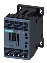
power contactor, AC-3e/AC-3, 7 A, 3 kW / 400 V, 3-pole, 24 V AC, 50/60 Hz, auxiliary contacts: 1 NO, spring-loaded terminal, size: S00,
