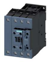
contactor AC-1, 60 A, 400 V / 40  $^{\circ}$ C, 4-pole, 110 V AC, 50 Hz, auxiliary contacts: 1 NO + 1 NC, screw terminal, size: S2
