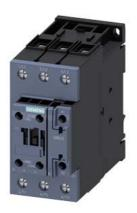
power contactor, AC-3e/AC-3, 41 A, 18.5 kW / 400 V, 3-pole, 110 V AC, 50 Hz / 120 V, 60 Hz, auxiliary contacts: 1 NO + 1 NC, screw terminal, size: S2, upright mounting position
