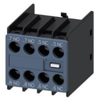
auxiliary switch, on the front, 2 NO + 2 NC, 22 U, .7/.8, .7/.8, .5/.6, .5/.6, current path: 1 NO (leading), 1 NO (leading), 1 NC (lagging), 1 NC (lagging), screw terminal, for contactors 3RT2 and contactor relays 3RH2
