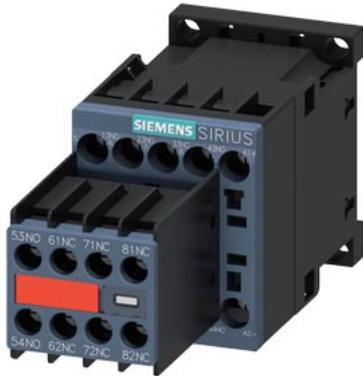
contactor relay, 5 NO + 3 NC, 24 V DC, size S00, screw terminal, captive auxiliary switch
