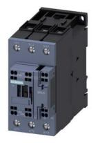
power contactor, AC-3e/AC-3, 80 A, 37 kW / 400 V, 3-pole, 48 V AC, 50 Hz, auxiliary contacts: 1 NO + 1 NC, main circuit: screw terminal, control and auxiliary circuit: spring-loaded terminal, size: S2
