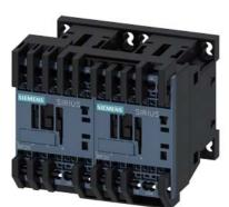
reversing contactor assembly, AC-3e/AC-3, 7 A, 3 kW / 400 V, 3-pole, 24 V DC, spring-loaded terminal, electrical and mechanical interlock
