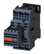
power contactor, AC-3e/AC-3, 32 A, 15 kW / 400 V, 3-pole, 230 V AC, 50/60 Hz, with plugged-in varistor, auxiliary contacts: 2 NO + 2 NC, spring-loaded terminal, size: S0, captive auxiliary switch
