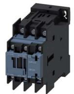
traction contactor, AC-3e/AC-3, 17 A, 7.5 kW / 400 V, 3-pole, 72 V DC, 0.7-1.25\* Us, electronic drive, with integrated varistor, auxiliary contacts: 1 NO + 1 NC, ring cable lug connection, size: S0
