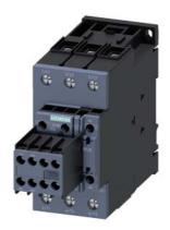
power contactor, AC-3e/AC-3, 41 A, 18.5 kW / 400 V, 3-pole, 220 V AC, 50/60 Hz, auxiliary contacts: 2 NO + 2 NC, screw terminal, size: S2, removable auxiliary switch
