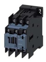
traction contactor, AC-3e/AC-3, 17 A, 7.5 kW / 400 V, 3-pole, 24 V DC, 0.7-1.25\* Us, electronic drive, with integrated varistor, auxiliary contacts: 1 NO + 1 NC, ring cable lug connection, size: S0
