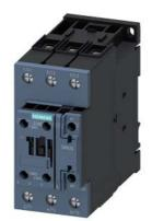
traction contactor, AC-3e/AC-3, 51 A, 22 kW / 400 V, 3-pole, 110 V DC, 0.7-1.25\* Us, electronic drive, with integrated varistor, auxiliary contacts: 1 NO + 1 NC, screw terminal, size: S2
