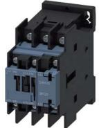
power contactor, AC-3e/AC-3, 38 A, 18.5 kW / 400 V, 3-pole, 460 V AC, 60 Hz, auxiliary contacts: 1 NO + 1 NC, ring cable lug connection, size: S0  $\,$
