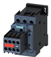
power contactor, AC-3e/AC-3, 32 A, 15 kW / 400 V, 3-pole, 110 V AC, 50 Hz / 120 V, 60 Hz, with plugged-in varistor, auxiliary contacts: 2 NO + 2 NC, screw terminal, size: S0, captive auxiliary switch
