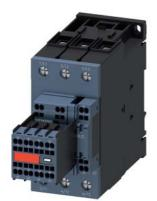
power contactor, AC-3e/AC-3, 80 A, 37 kW / 400 V, 3-pole, 230 V AC, 50/60 Hz, with plugged-in varistor, auxiliary contacts: 2 NO + 2 NC, main circuit: screw terminal, control and auxiliary circuit: spring-loaded terminal, size: S2, captive auxiliary switch
