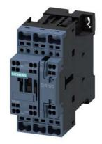
power contactor, AC-3e/AC-3, 25 A, 11 kW / 400 V, 3-pole, 220 V DC, auxiliary contacts: 1 NO + 1 NC, spring-loaded terminal, size: S0  $\,$
