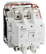
Mechanically held lighting contactor, Contactor amp rating 100A, 0 N.C. / 3 N.O. poles, 220VAC 50HZ/240VAC 60HZ coil, Non-combination type, Enclosure NEMA type (open), No enclosure
