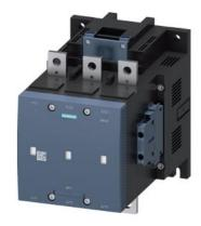
vacuum contactor AC-3e/AC-3 400 A, 200 kW / 400 V, 3-pole, Uc: 23-26 V AC(50-60 Hz) / DC drive: conventional auxiliary contacts 2 NO + 2 NC main circuit: busbar control and auxiliary circuit: screw terminal
