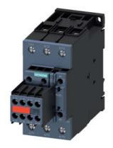
power contactor, AC-3e/AC-3, 51 A, 22 kW / 400 V, 3-pole, 110 V AC, 50 Hz / 120 V, 60 Hz, with plugged-in varistor, auxiliary contacts: 2 NO + 2 NC, screw terminal, size: S2, captive auxiliary switch
