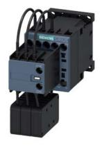
capacitor contactor, AC-6b 12.5 kVAr, / 400 V, 3-pole, 110 V DC, auxiliary contacts: 2 NC, screw terminal, size: S00  $\,$
