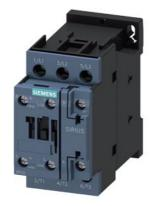
power contactor, AC-3e/AC-3, 32 A, 15 kW / 400 V, 3-pole, 48 V AC, 50/60 Hz, auxiliary contacts: 1 NO + 1 NC, screw terminal, size: S0
