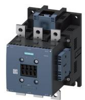
power contactor, AC-3e/AC-3 265 A, 132 kW / 400 V Uc: 24 V DC x (0.7-1.25) PLC input 24-110 V DC 3-pole, auxiliary contacts 2 NO + 2 NC drive: electronic main circuit: busbar control and auxiliary circuit: spring-loaded terminal extended rated condition railroad IEC 60077
