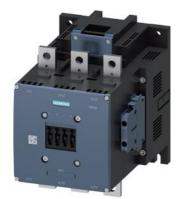
power contactor AC-1 690 A / 690 V / 40  $^\circ$ C 3-pole, Uc: 575-600 V AC(50-60 Hz) / DC drive: conventional auxiliary contacts 2 NO + 2 NC main circuit: busbar control and auxiliary circuit: screw terminal
