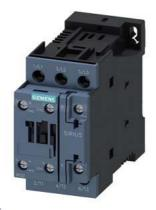
power contactor, AC-3e/AC-3, 25 A, 11 kW / 400 V, 3-pole, 24 V DC, with plugged-in varistor, auxiliary contacts: 1 NO + 1 NC, screw terminal, size: S0, upright mounting position
