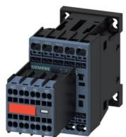
power contactor, AC-3e/AC-3, 16 A, 7.5 kW / 400 V, 3-pole, 24 V DC, auxiliary contacts: 2 NO + 2 NC, spring-loaded terminal, size: S00, captive auxiliary switch
