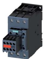
power contactor, AC-3e/AC-3, 41 A, 18.5 kW / 400 V, 3-pole, 230 V AC, 50 Hz, auxiliary contacts: 2 NO + 2 NC, screw terminal, size: S2, captive auxiliary switch
